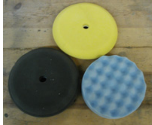
Figure 4 - Large buffer pads – black, yellow, and blue (very soft, on the right)
