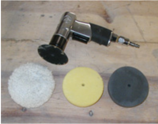
Figure 3 - 3-inch polishing machine & pads. The wool pad on the left is more aggressive and is only used where spots require more aggressive treatment and there is sufficient paint thickness
