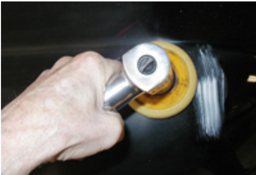
Figure 5 - Apply compounds sparingly as shown using a brush. Then, move the buffing pad into the compound at slow speed.
